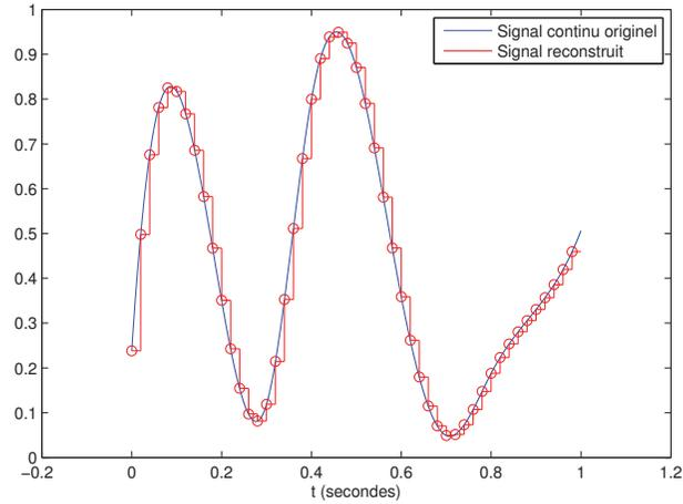
$F_s = 50$  Hz,  $T_s = 0.02$  secondes. Reconstruction encore imparfaite.
