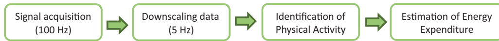
Fig. 2. Illustration of the data treatment chain from the motion sensor signal acquisition to the identification of the subject's posture, hence its PA, followed by the calculation of the estimated EE.
