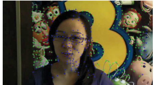
Fig. 1. Example on the close_person video (frame 100). All trajectories belonging to the time-window of interest are projected in the (\mathbf{u}^x, \mathbf{u}^y) plane. The majority of the contributions aggregate around the red point (mode of the 2D histogram). When selecting only feature points close to this mode (green points), we retrieve feature points from the background that are only corrupted by camera motion. On the contrary feature points far from the mode (blue points) correspond either to the moving woman or to spurious feature points.
